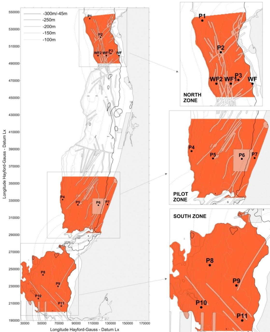
Figure 7 - Simulation grid zones for the offshore wind resource assessment and for the wind farm energy production estimates with the identification of the constraints exclusion areas.
