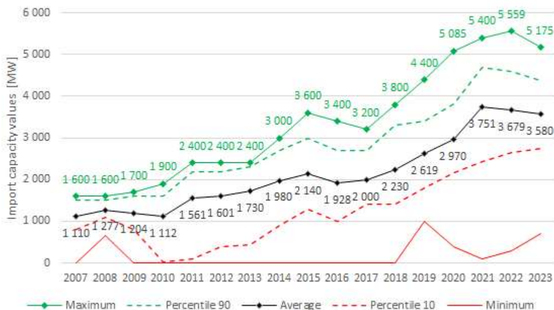
Figure 2 2 - Evolution of interconnection capacity available for commercial purposes - Imports
