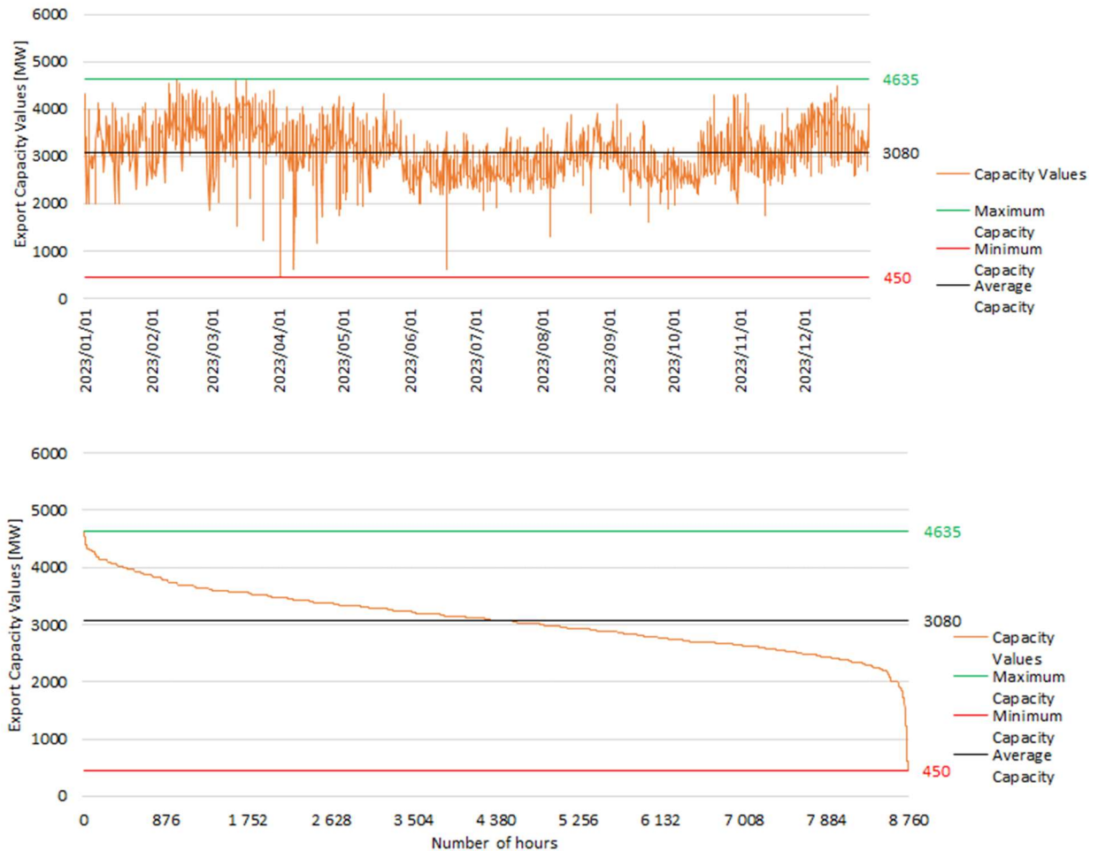
Figure 2 6 - Hourly values of interconnection capacity available for commercial purposes in 2023 - Exports
