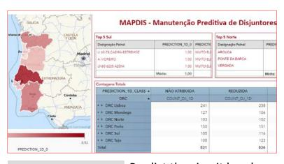
9.000 Circuit breakers Predict the circuit breakers with highest probability of failure in the next command and prioritize maintenance by risk. Estimate yearly savings: 0,5M€ - 1M€
