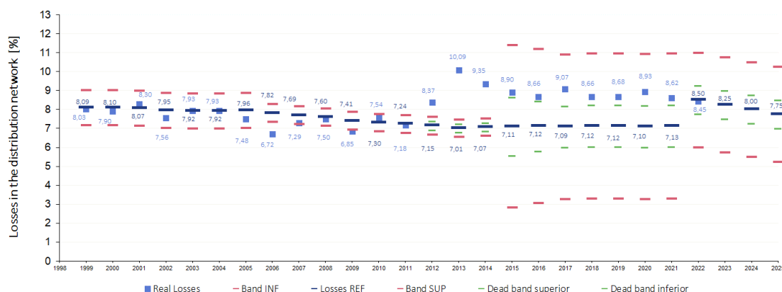
Figure 18 – Evolution of verified losses in distribution networks in the input reference
