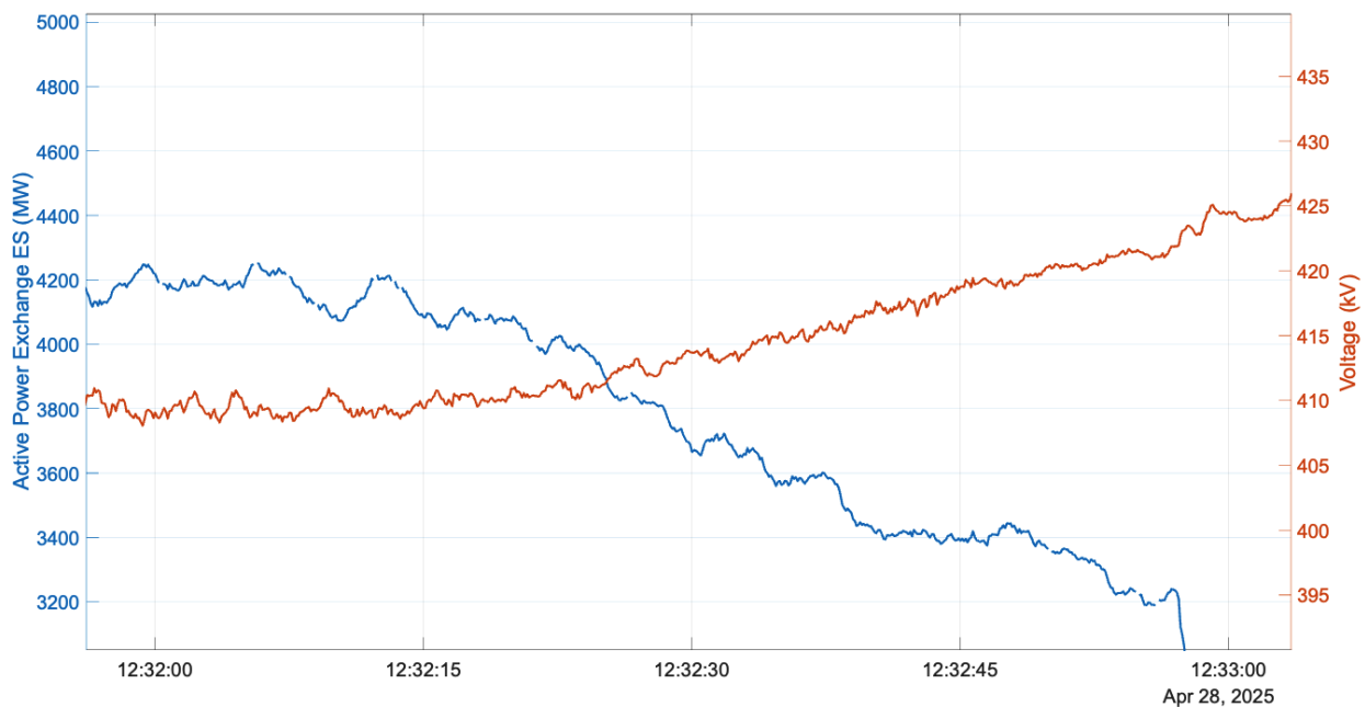
Figure 11: Voltage evolution at the Carmona substation and Spain's net active power exchange position in the minute before the blackout (source: Red Eléctrica PMU data)
