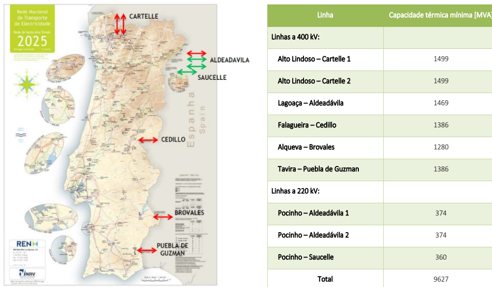
Figure 11 – Interconnection lines between Portugal and Spain and the thermal capacities of the lines 87
